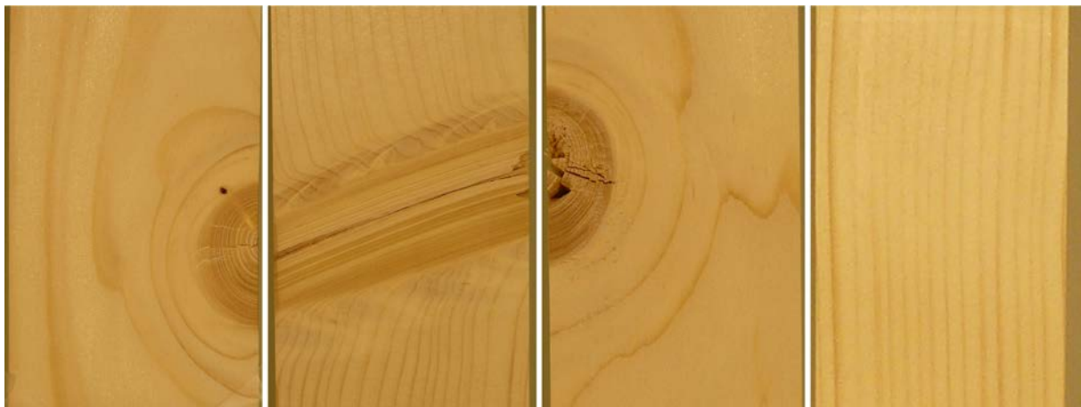
Figure 2.8: A knot seen from all four sides of a wood specimen 45 x 45 mm in square section (Photo Bertil Enquist).
