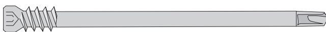
Figure 4.19: Special fastener designed for steel-to-timber joints enabling drilling the hole and mounting the fastener in one working moment.
