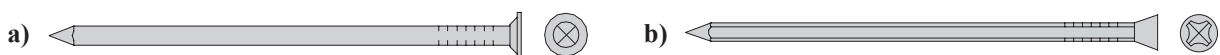
Figure 4.1: Examples of nails. a) Round, smooth nail, b) grooved, smooth nail (here a brad).
